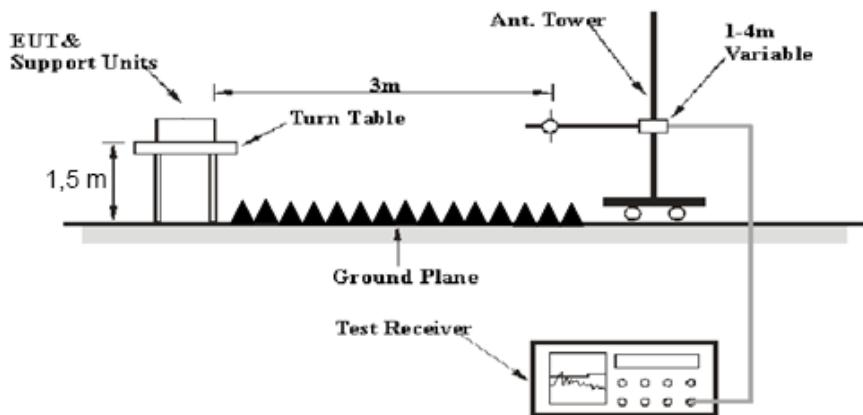
The radiated emission tests were performed in the 3 meters chamber test site, using the setup accordance with the ANSI C63.10-2013. The specification used was the FCC 15.209, and FCC 15.247 limits.
