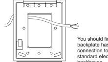
You should find that the backplate has holes for connection to most standard electrical backboxes.
