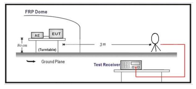
Below 1GHz Test Setup:
