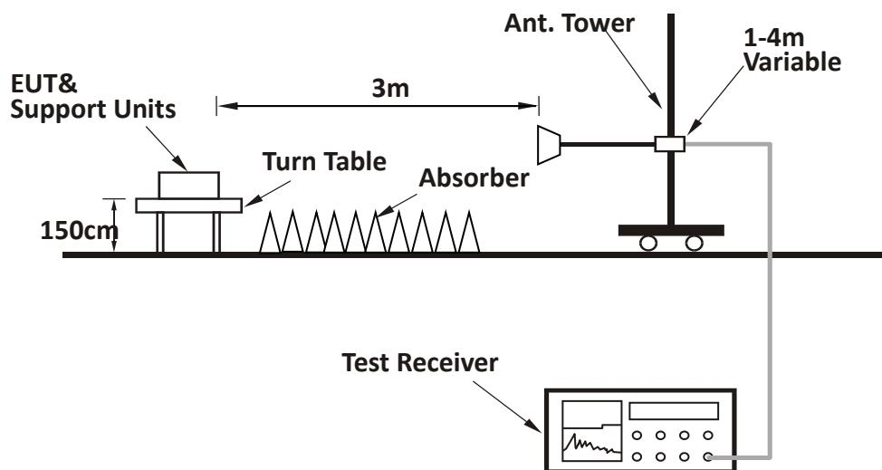
**TEST REPORT****7.4 Test Results of Radiated Emissions**
