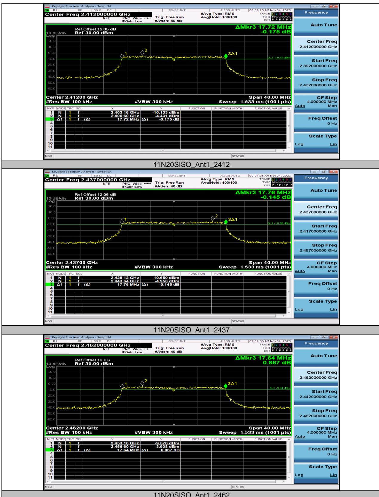
**TEST REPORT****Occupied Channel Bandwidth****Test Result**
