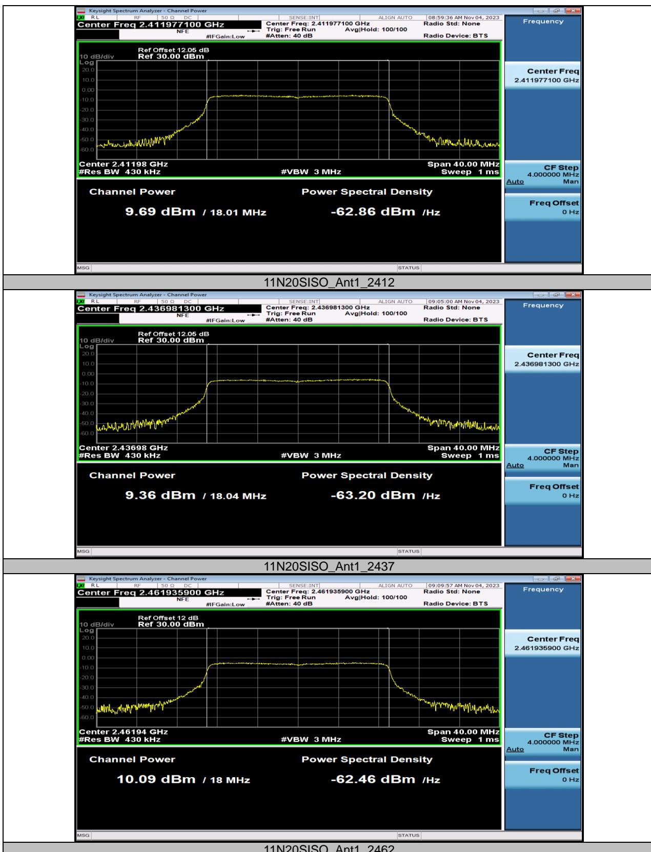
**TEST REPORT****Maximum power spectral density****Test Result**
