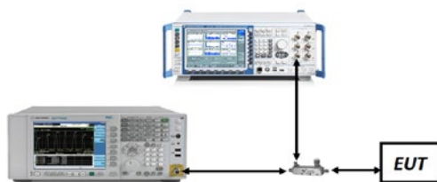
Figure 7-1. Test Instrument & Measurement Setup
