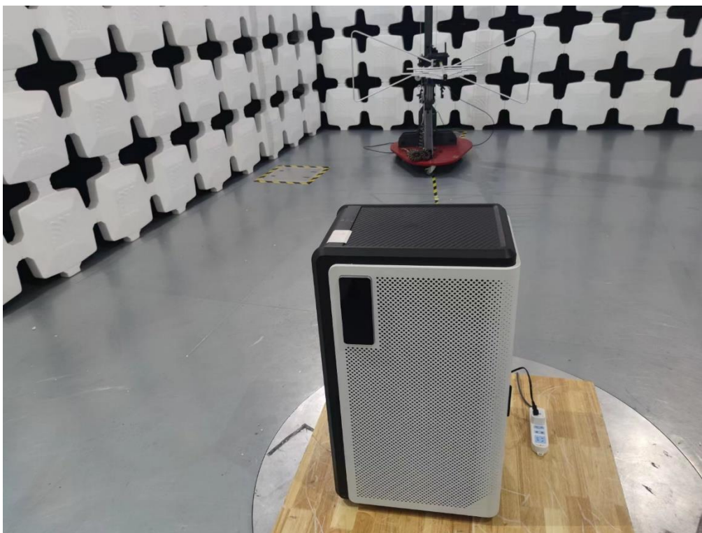
Radiated Emission test below 1GHz
