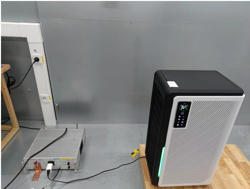
Radiated Emission test below 1GHz
