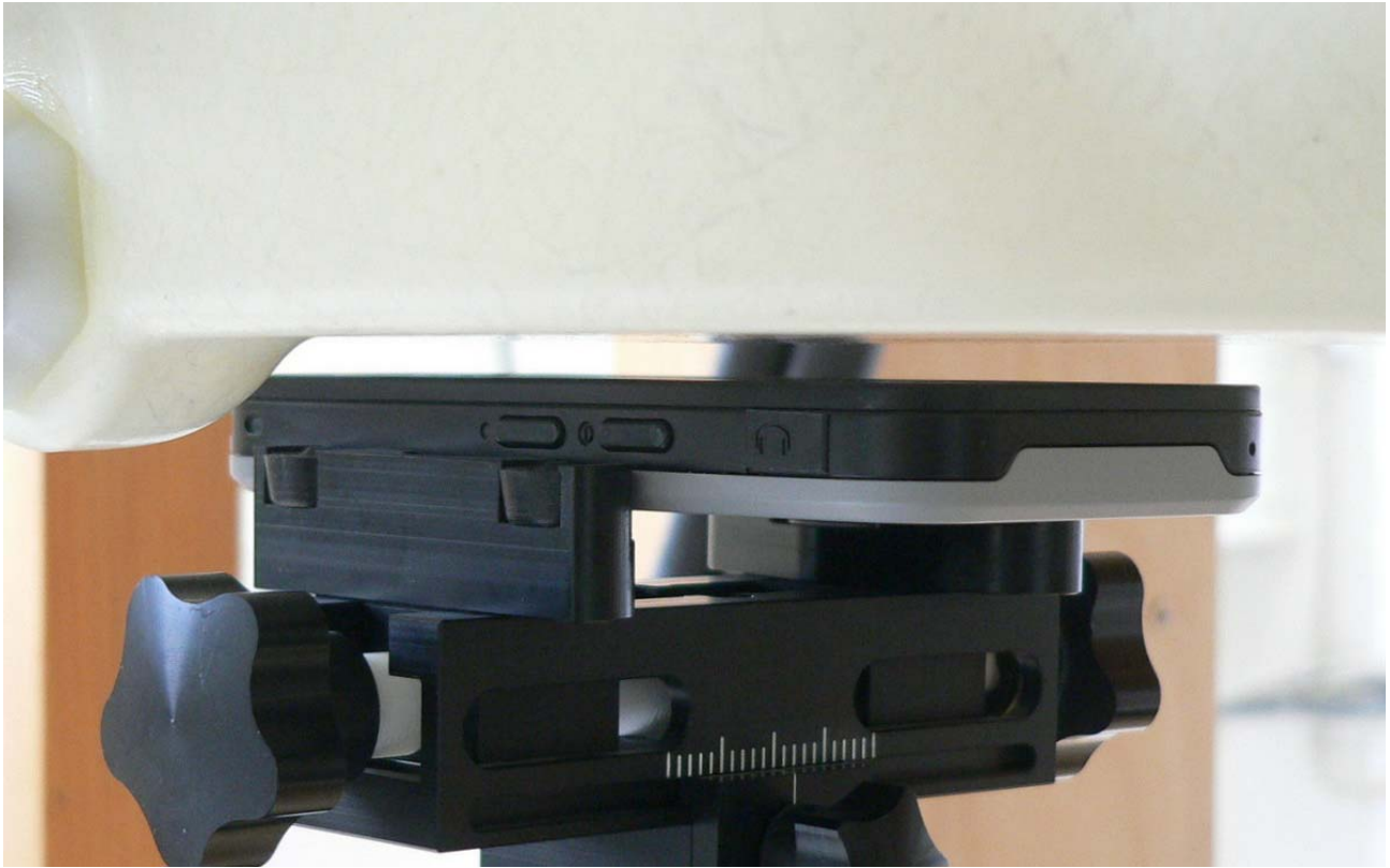
Fig. 18: Front side towards the phantom, 5mm distance.
