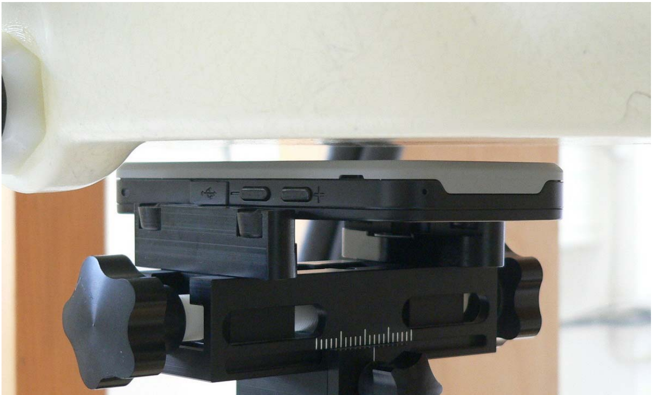
Fig. 19: Back side towards the phantom, 5mm distance.
