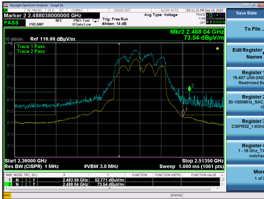
Graph 8: Radiated Upper Band Edge Plot n mode (40)
