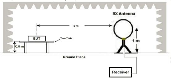
2. Radiated Emission Test-Up Frequency 30MHz~1GHz
