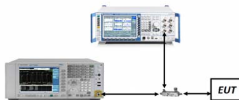
Figure 7-1. Test Instrument & Measurement Setup
