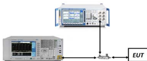
Figure 7-3. Test Instrument & Measurement Setup
