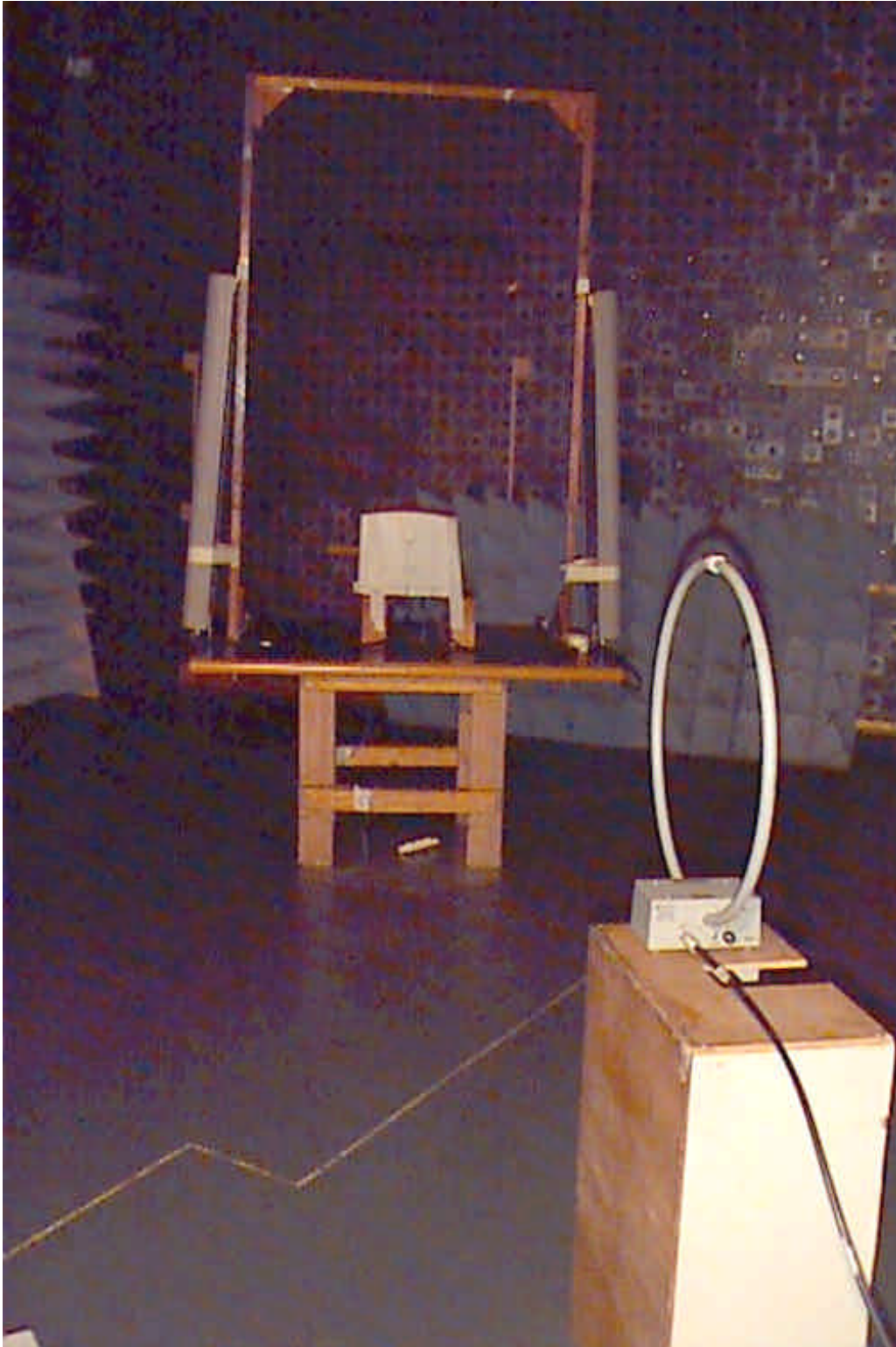
Photograph No.2 Radiated emissions measurement setup in the anechoic chamber with loop antenna
