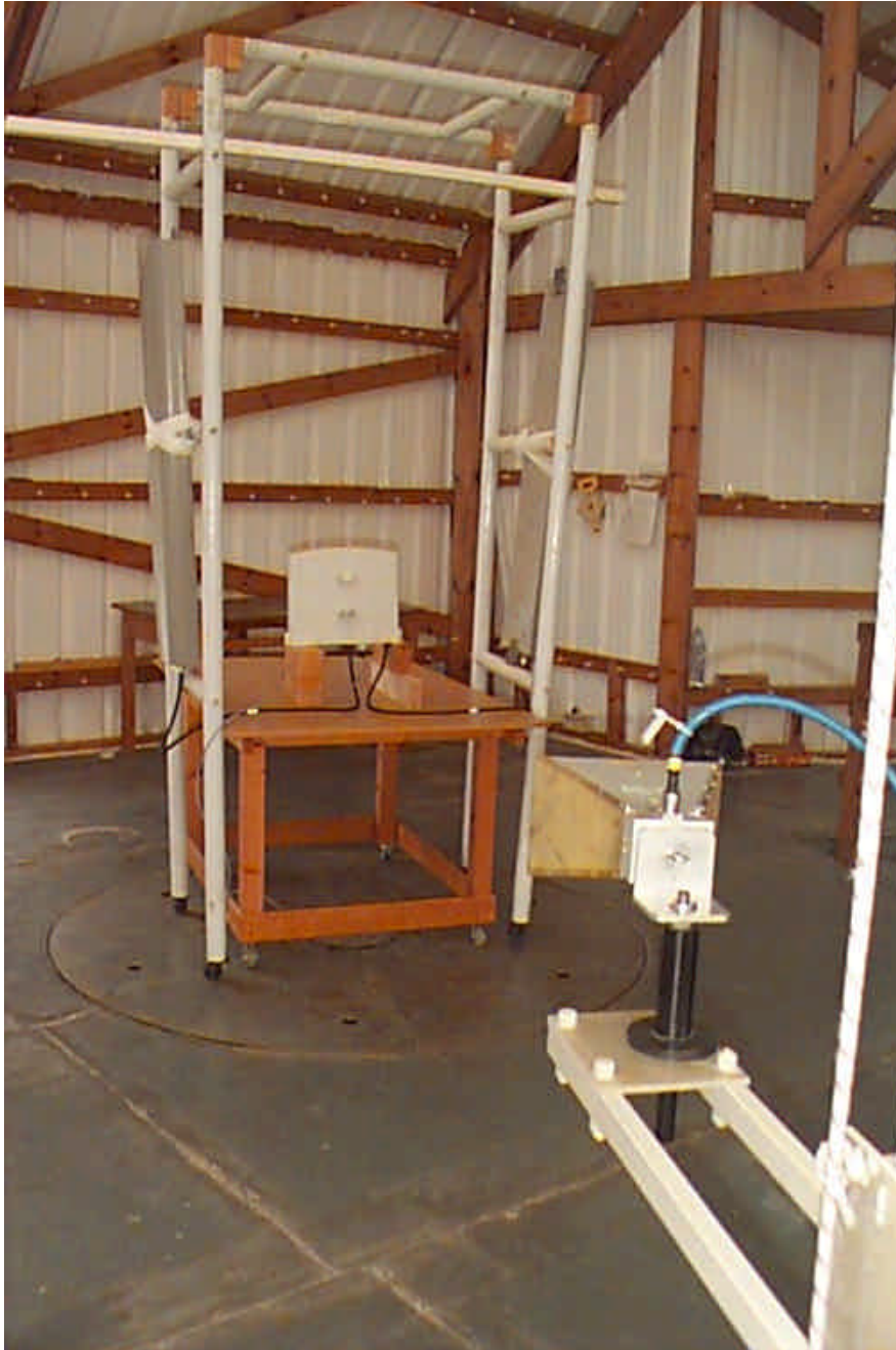
Photograph No.5 Radiated emissions measurement setup at the OATS with double ridged guide antenna
