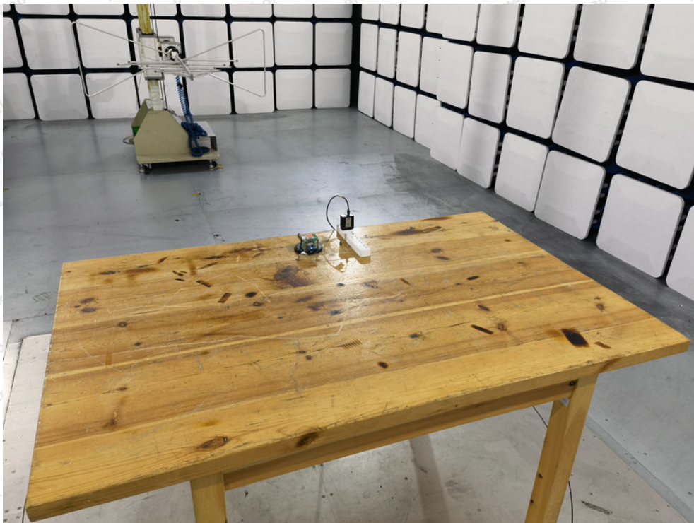
Photo of Radiation Emission Test
