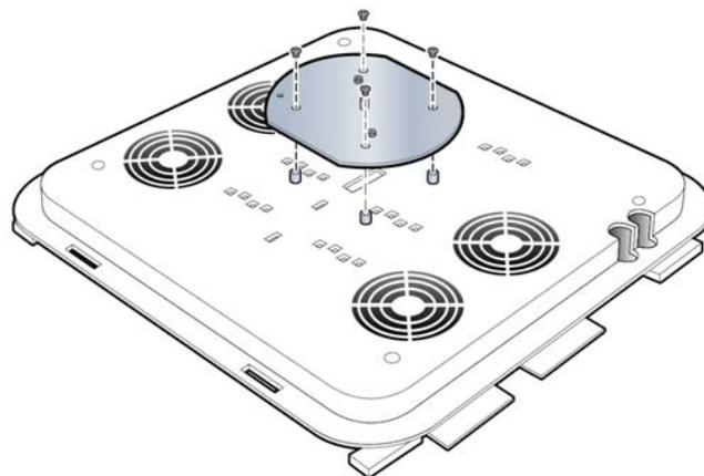
9 Mount the Radio Point on the octagon box plate.
