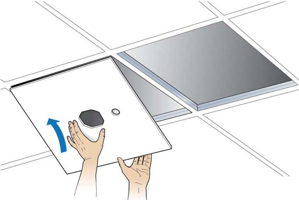
6 Install the drop rail/octagon box assembly over the modified tile.
