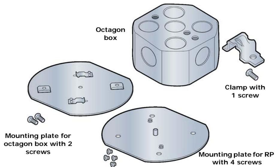
Mounting the Radio Point (RP) in the flown configuration requires the following hardware provided by the system integrator:
