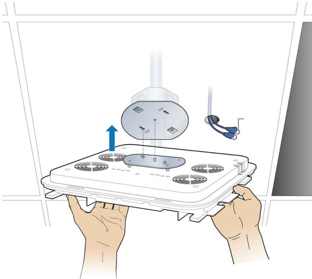
**10** Secure Radio Point to plate.
