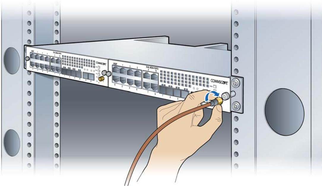
11 Connect the Ethernet or fiber optic cable to the appropriate port.
