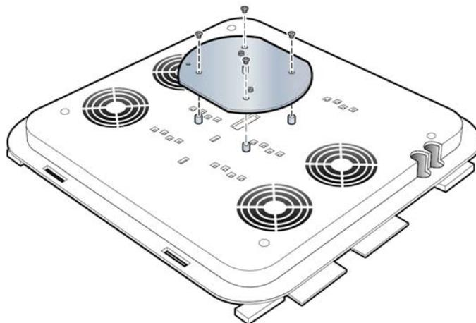
5 Attach the Radio Point to the octagon box mounting plate.
