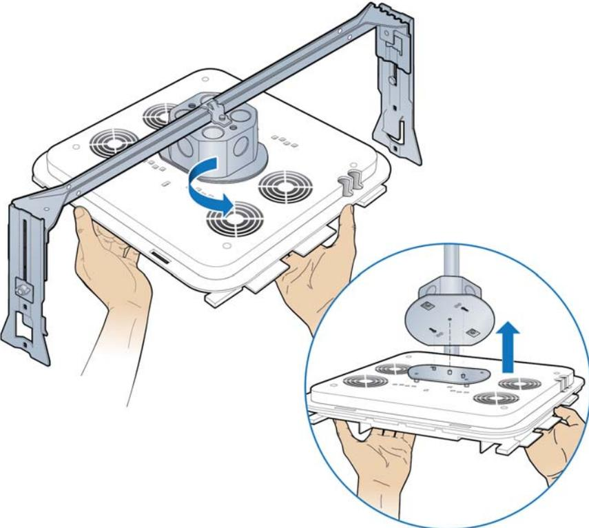
6 Install drop rail above the ceiling tile.
