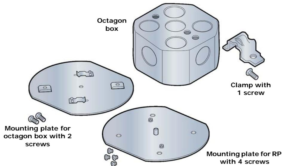
Mounting the Radio Point (RP) above or on the ceiling tile requires the following hardware provided by the system integrator:
