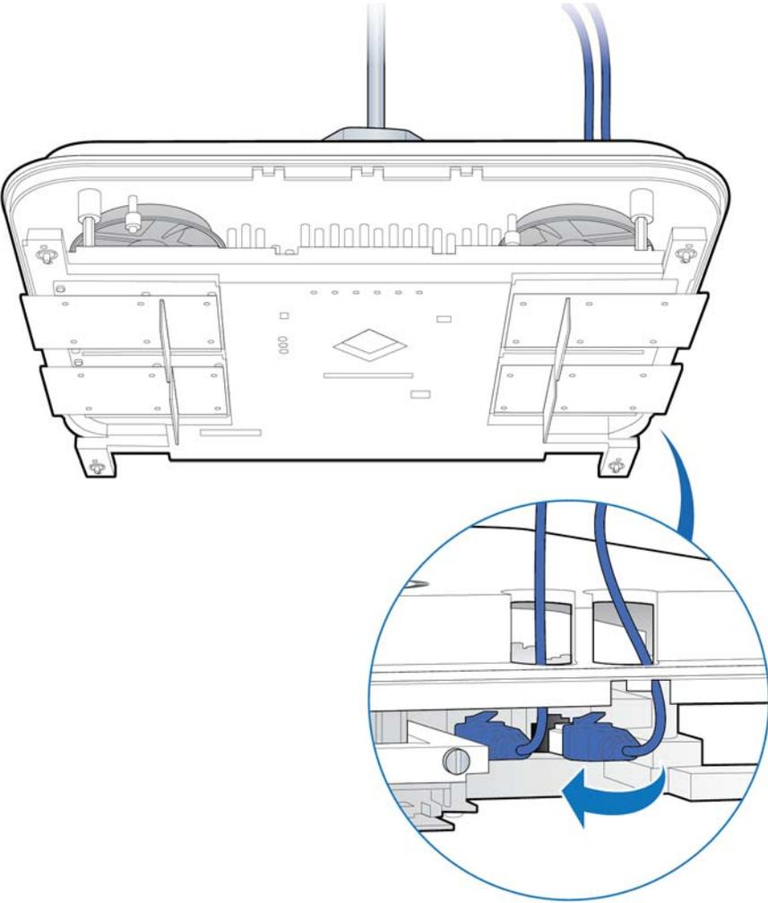
**8** Attach the plastic cover to the Radio Point.
