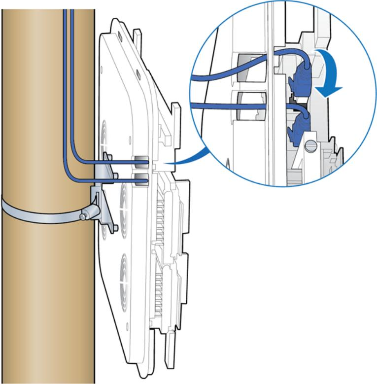
5 Attach the plastic cover to the Radio Point.
