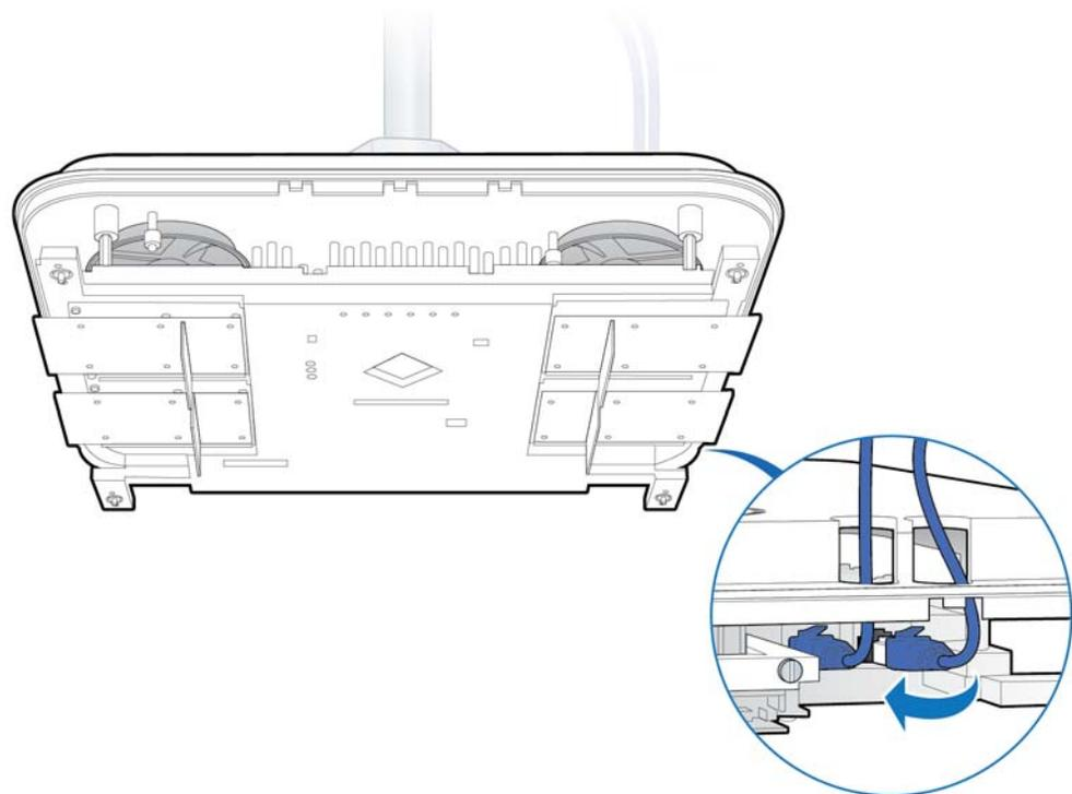
12 Attach the plastic cover to the Radio Point.
