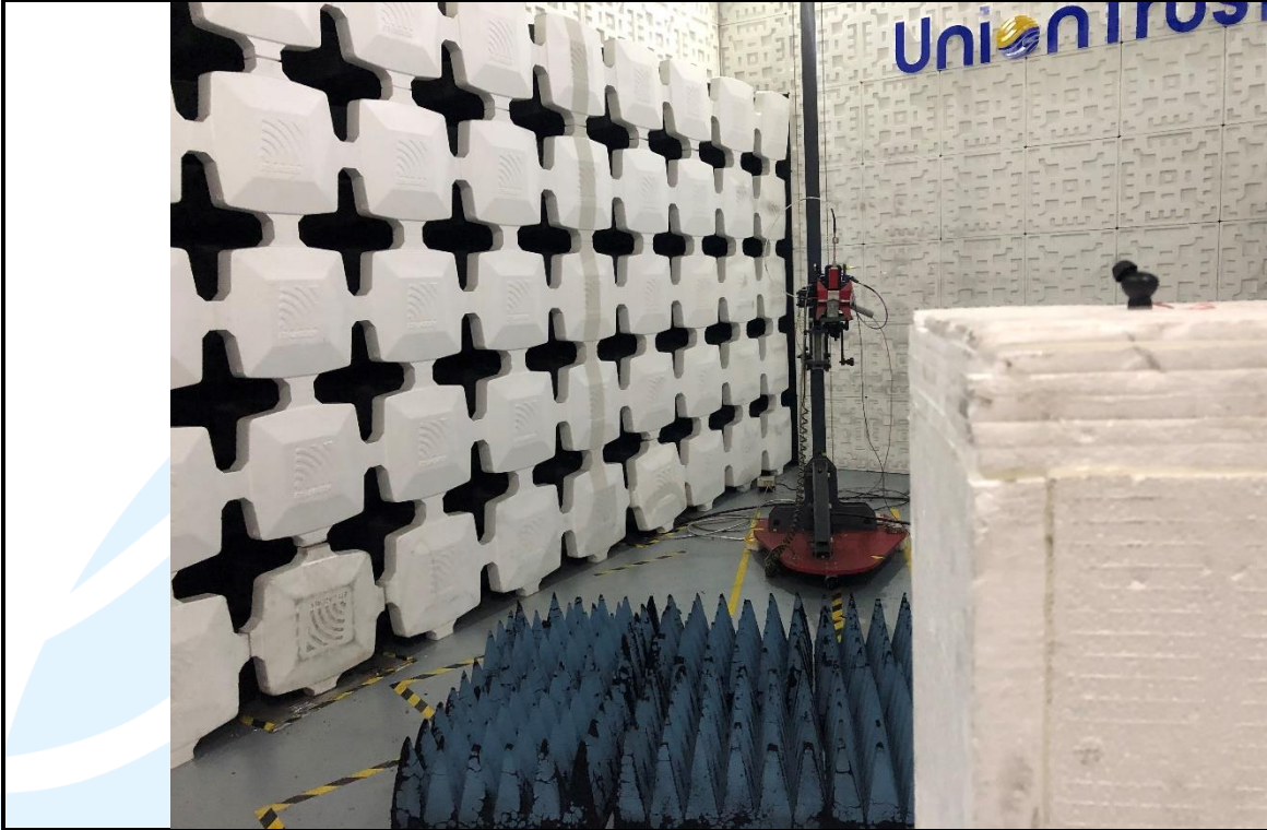
Radiated emission Test Setup (Above 1 GHz) -Left
