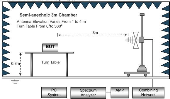
(C) Radiated Emission Test-Up Frequency Above 1GHz
