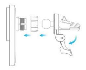
1. Remove the ball joint fastener from the wireless car charger by rotating it
