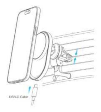
4. Connect the other charging cable end to the USB-C port of a USB car adapter, or a USB car adapter that fits into the cigarette lighter socket.
