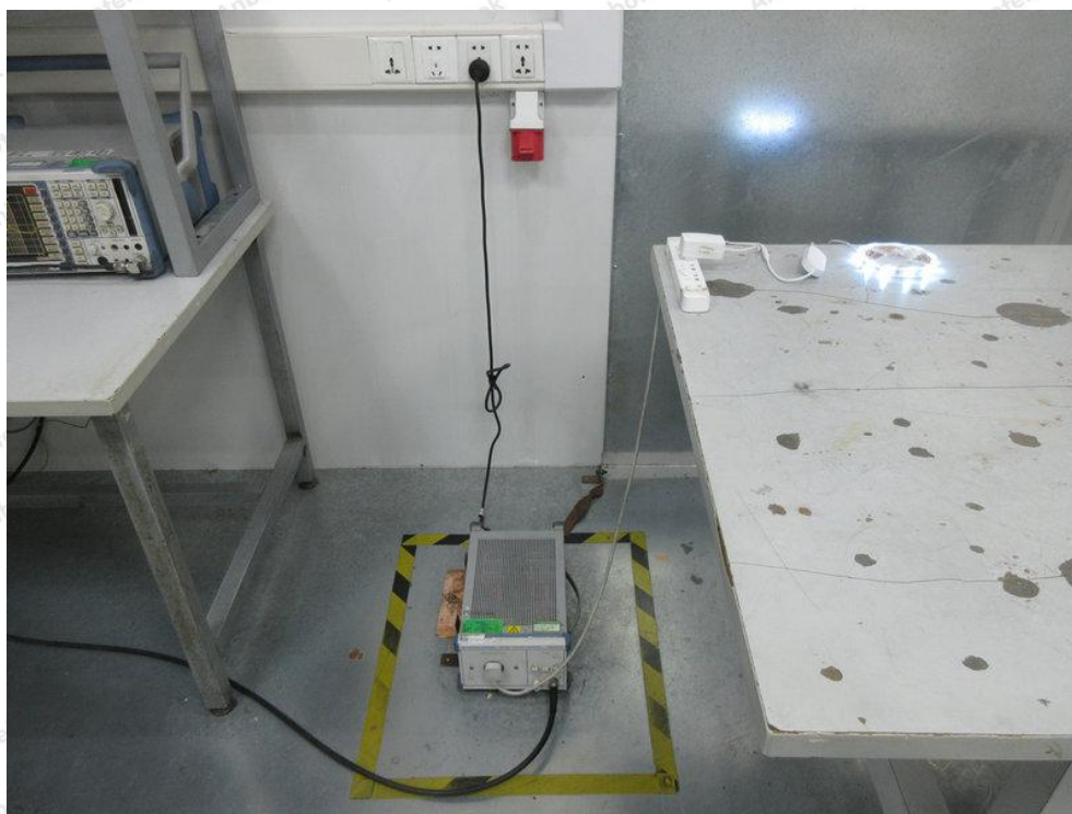
Photo of Conducted Emission Measurement
