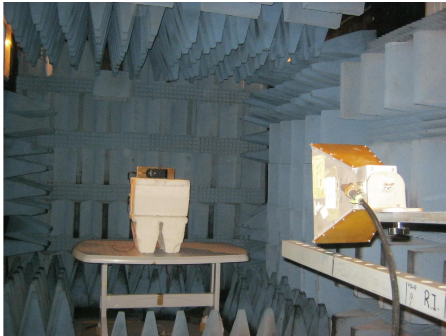
Figure 8. Radiated Emission Test, 1-18GHz
