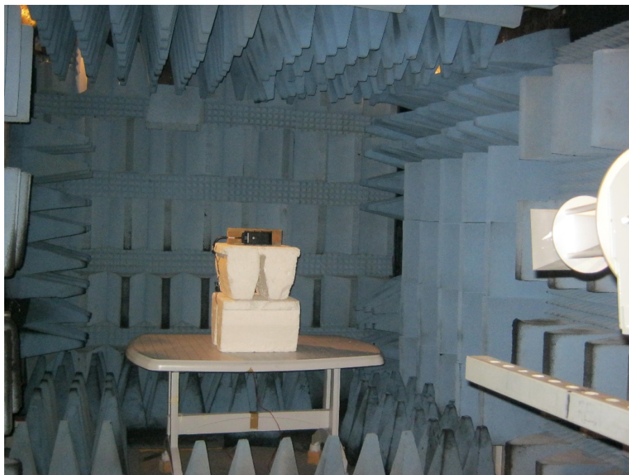
Figure 9. Radiated Emission Test, 18-26.5GHz
