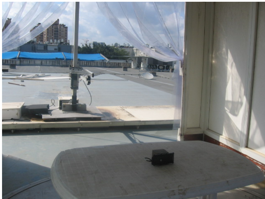
Figure 7. Radiated Emission Test, 200-1000MHz
