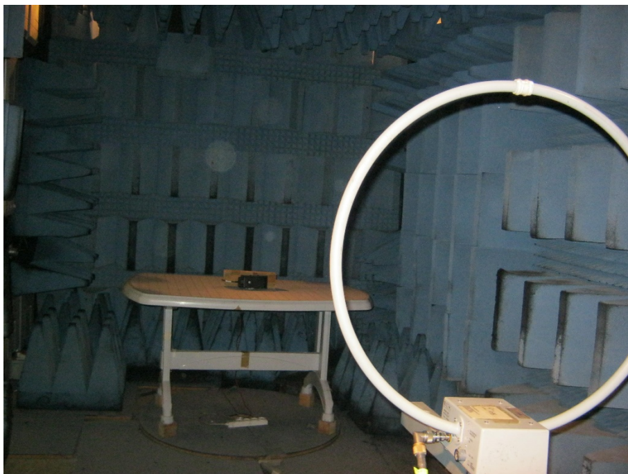
Figure 5. Radiated Emission Test, 0.009-30MHz
