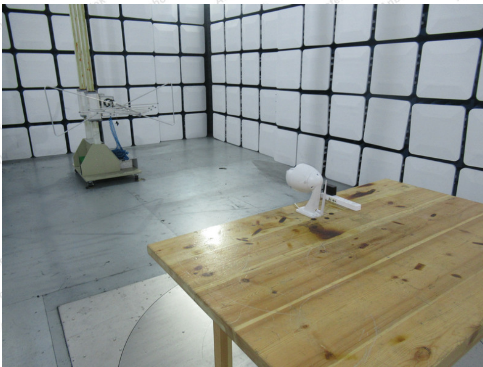
Photo of Radiation Emission Test
