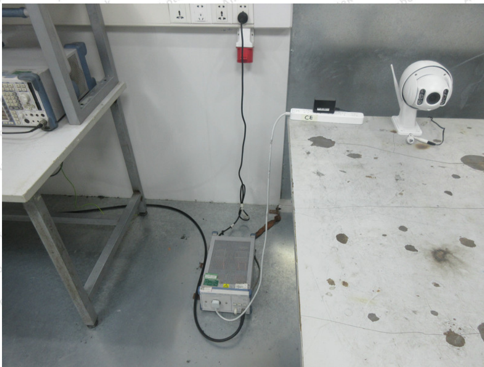
Photo of Conducted Emission Measurement
