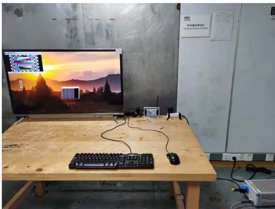
Photo of Conducted Emission Measurement
