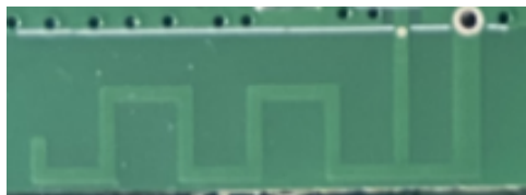
Photo of Antenna
