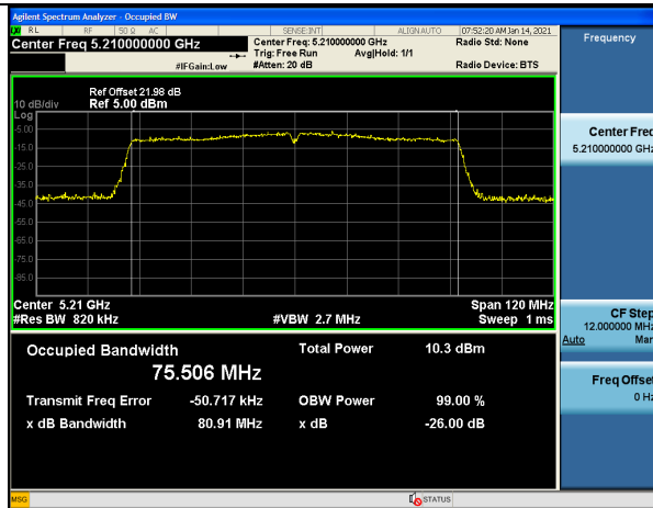
802.11ac_VHT80 UNII 2C BAND 26dB Bandwidth(CH 138)
