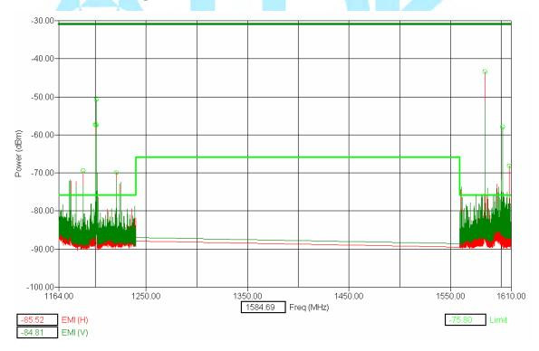
Limit line is 47 CFR, Part 15 subpart C
