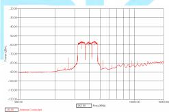
Terminated antenna port measurements made with 1 MHz RBW  $\!$  / 3 MHz VBW at 1 meter distance
