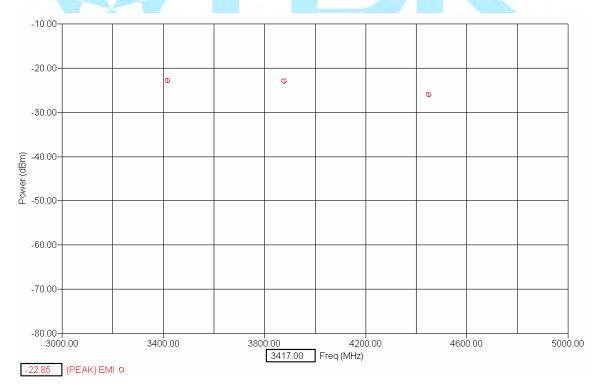
Measurements made with 5 MHz RBW / 5 MHz VBW at 3 meter distance.
