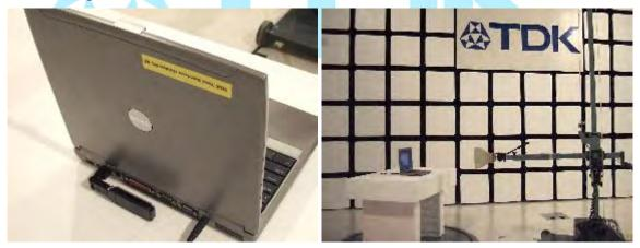
Test Configuration 2. 30 MHz to 960 MHz
