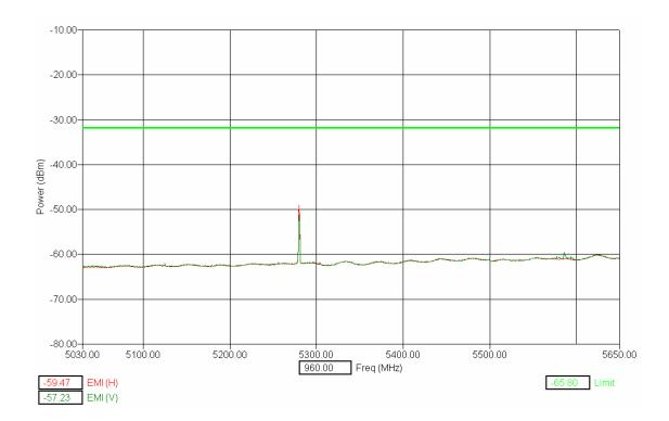
Measurements made with 1MHz RBW and 3MHz VBW at 1-meter distance
