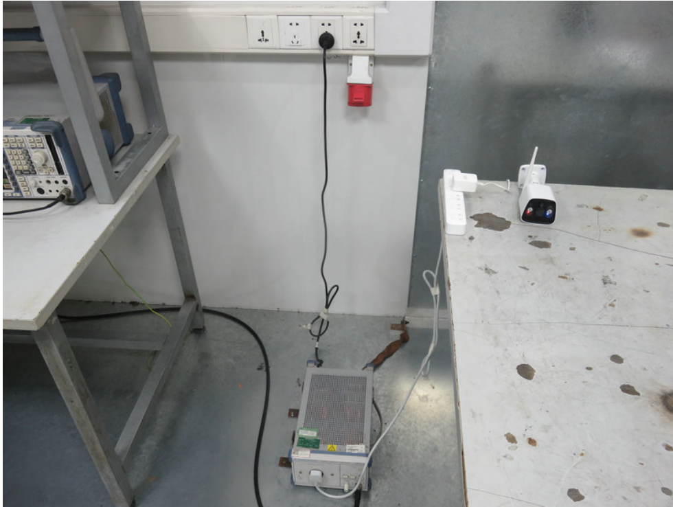
Photo of Conducted Emission Measurement
