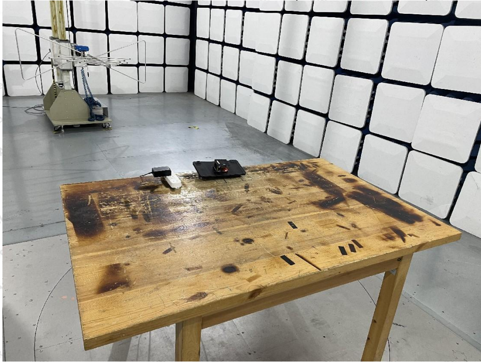
Photo of Radiation Emission Test (30MHz~1000MHz)
