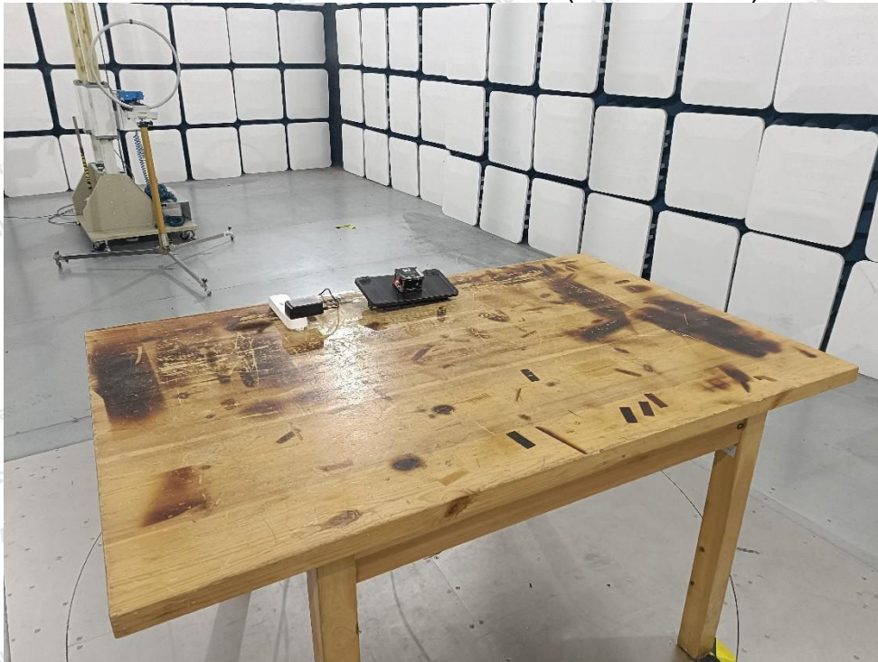
Photo of Radiation Emission Test (below 30MHz)
