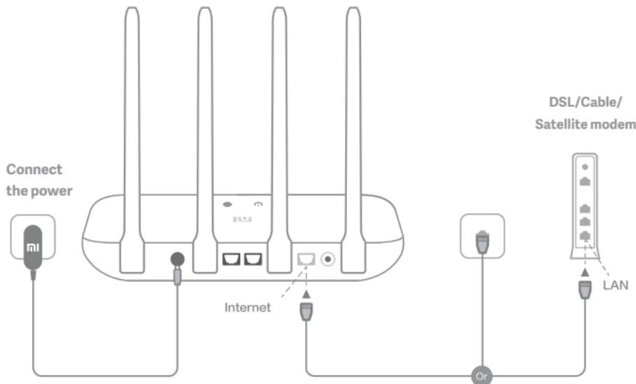
**Power on the router, then connect the Internet (WAN) port to the DSL/Cable/satellite modem**
