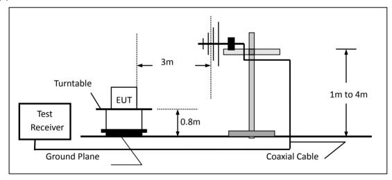
(c) For radiated emissions above 1000MHz
