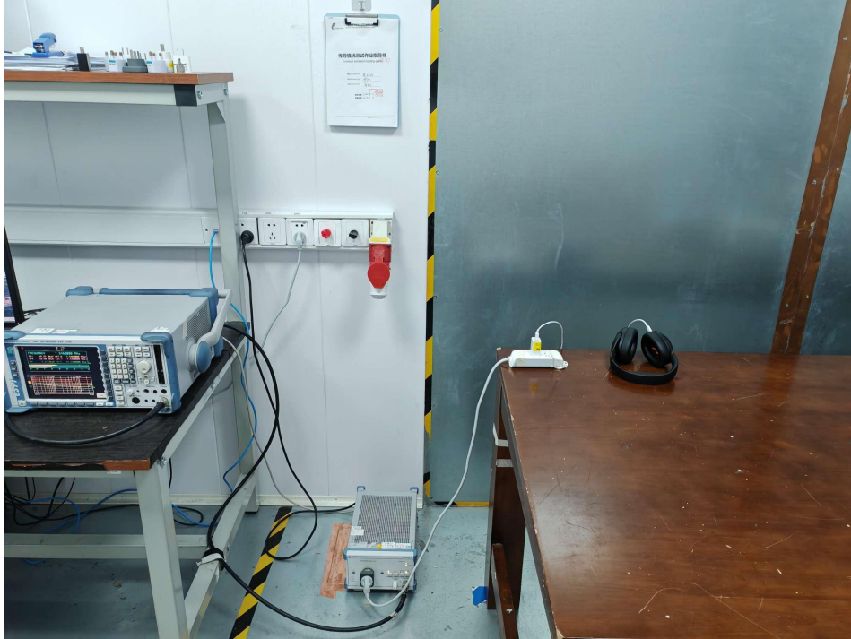
Conducted emissions at AC power line (150kHz-30MHz)
