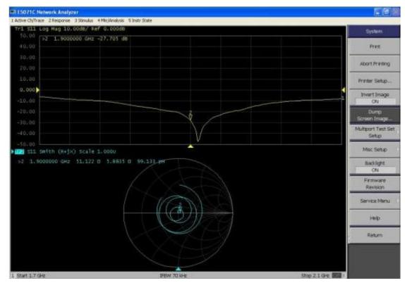
D1900V2, serial No. 5d162 Extended Dipole Calibrations
