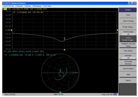
D2450V2, serial No. 818 Extended Dipole Calibrations
