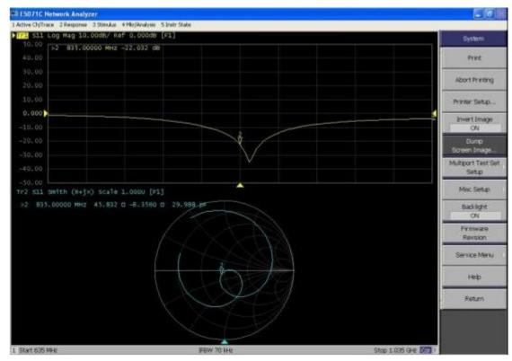
D835V2, serial No. 4d141 Extended Dipole Calibrations
