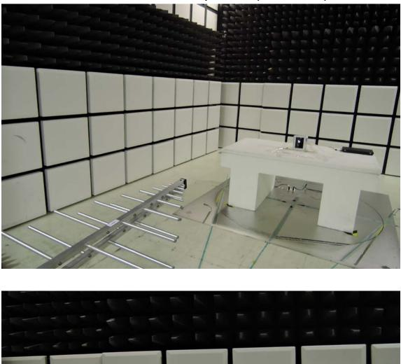
Radiated Emission Set up Photos (Below 1GHz)
