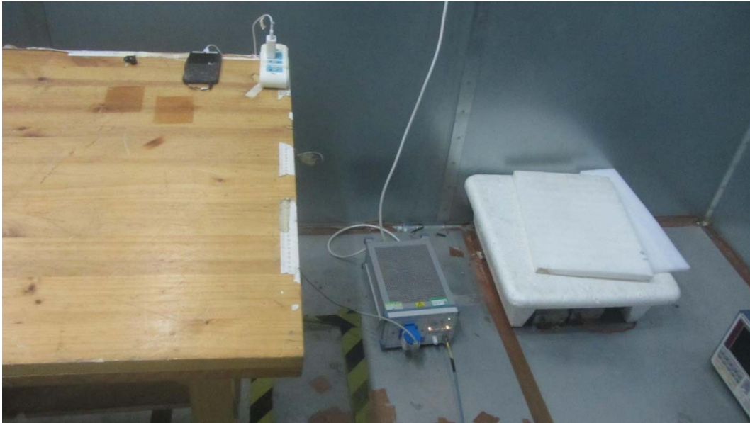
Picture 2 Conducted Emission Test Setup
