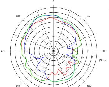
Average Gain And Peak Gain (On Azimuth Plane)
