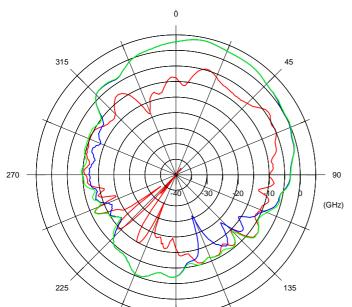
Average Gain And Peak Gain (On Azimuth Plane)
