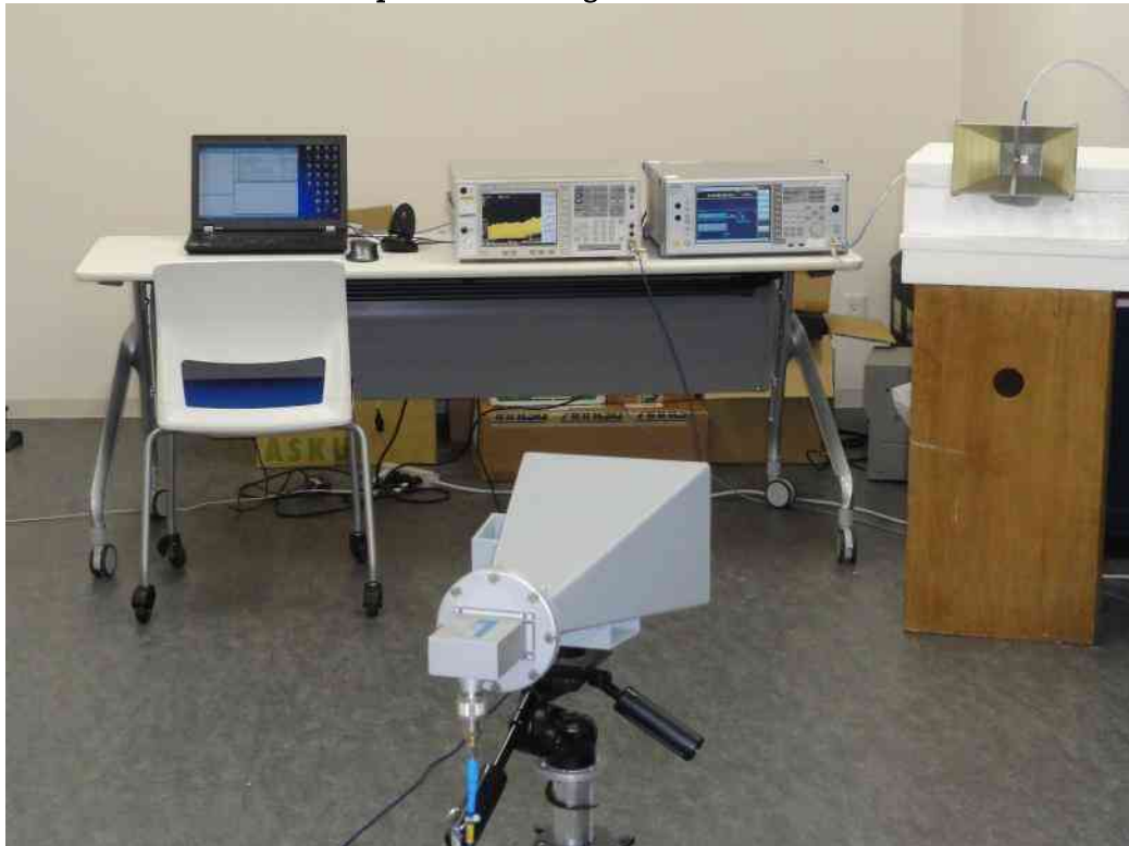
Test Setup for Generating the Radar Waveform
