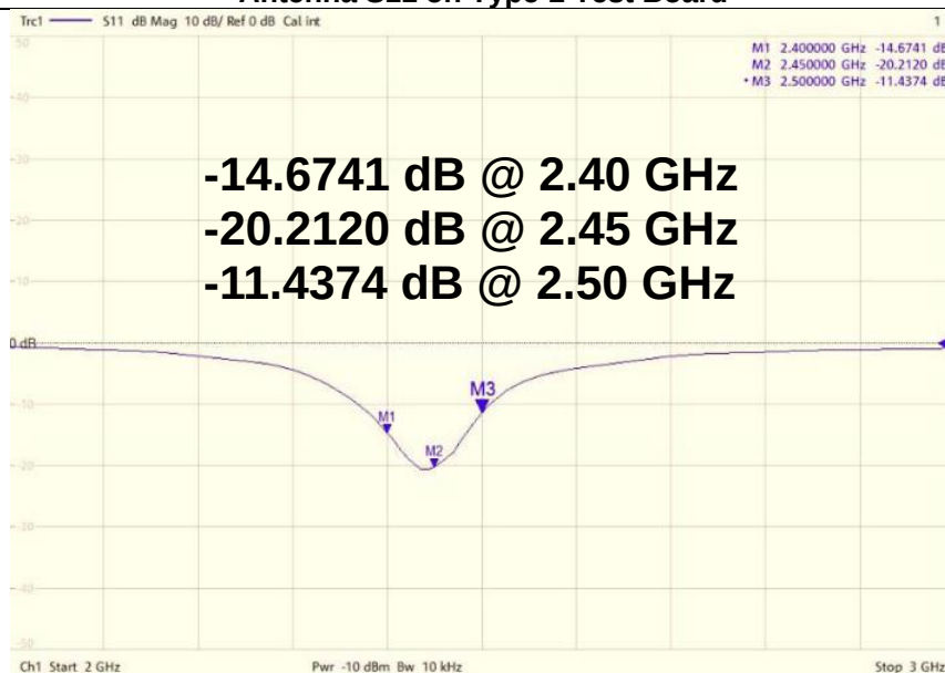
Antenna VSWR on Type-2 Test Board
