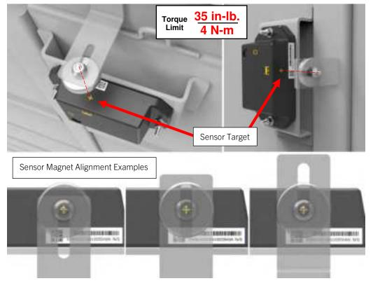
5. Once you have determined the best installation location and attachment method for your Radar S2 IS module and bracket assembly, place the module and bracket assembly in your desired installation location.
