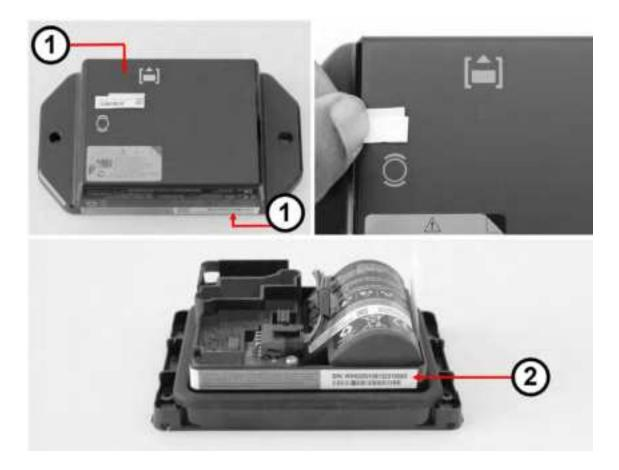
1. Once you have installed the module on the asset, create a record of the module-toasset-to-accessory pairing within the BlackBerry Mobile App by recording the asset identifier and scanning the module identifier for the BlackBerry Radar S2 IS and associated Radar H2M IS module.
