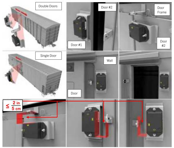
6. Once placement location is confirmed, use a pencil or marker to mark the outline of brackets for welding. NOTE: As an alternative to pencil marking, you may also use tape to mark the outline of the bracket position.
