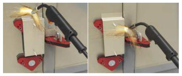
**Tip:** If you will use welding magnets in your installation, the use of heavy duty, three-axis welding magnets (with a face magnet) are recommended.
