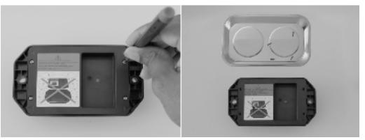
To separate the battery door from the outer housing—begin by inserting a flat screwdriver (3-7mm width) into a slot, marked with the arrows, and pry upwards. Complete the battery door removal by working your way around the door--inserting the screwdriver into the other slots and prying upwards, until the door is free.
