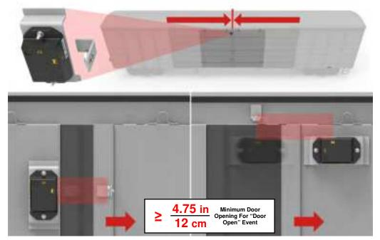
**IMPORTANT:** For accurate door event detection, ensure the distance between the Radar S2 IS module and Radar S2 IS Magnetic Sensor does not exceed 2" (5 cm).
