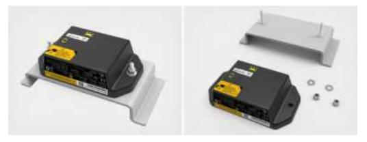
9. If you elected to remove the device while welding the bracket to your asset, ensure the bracket has cooled before re-attaching the Radar S2 IS to the to the bracket. Do not tighten the fastener beyond 35 in-lb. (4 N-m).
