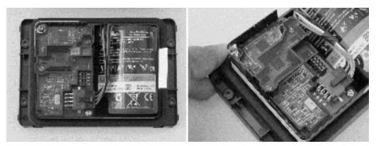
4. Fully install the battery door.
