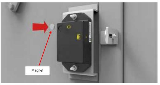
2. Place the magnet within the magnet recess on the front of the housing. Hold the magnet within the magnet recess for at least 5 seconds, then remove the magnet from the module. The module will reboot and reconnect to the previously paired Radar H2M IS module.
