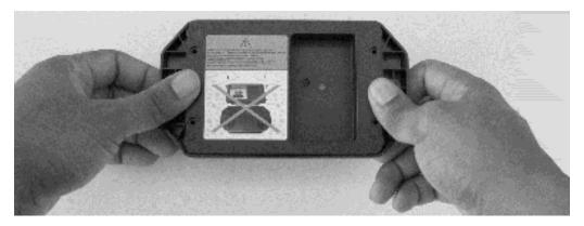
5. Using a Torx T10 screwdriver, install the screws to secure the battery door. **IMPORTANT:** Screw torque must be 2.6 in-lb (0.3 N-m).
