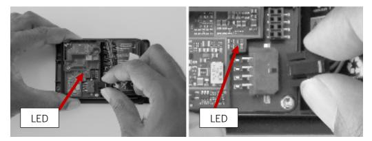
3. **IMPORTANT:** Prior to reassembly, closely inspect the clear encapsulant, over the circuit board, for any damage. If the encapsulant is damaged, replace the device.
