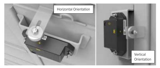
**IMPORTANT:** To provide more flexibility for aligning the center of the Radar S2 IS Magnetic Sensor magnet to the sensor target, the sensor magnet may be moved along the slot in the S2 IS Magnetic Sensor Bracket. To adjust the position of the sensor magnet, loosen the lock nut (if necessary), and reposition the sensor magnet into the desired location.
