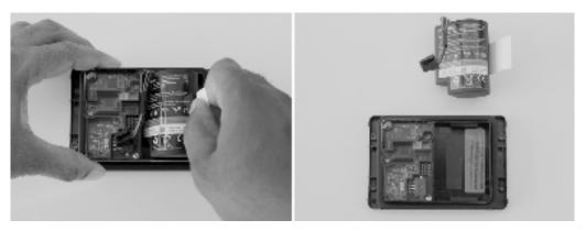
5. Without the battery installed, place the battery cover onto the module. Place the screws in the recess on the mounting flange and cover with tape. Leaving the screws uninstalled is recommended as an indicator to the recipient that there is no battery installed and must be installed before its next use. If no battery is installed, devices may be shipped in non-Dangerous Goods packaging.
