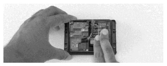
2. Connect the battery cable to the battery connector. The LED will blink to indicate the module is active. NOTE: It can take between 10-15 seconds for the blink sequence to begin. Please be patient. Once you see the LED blink, continue to the next step.
