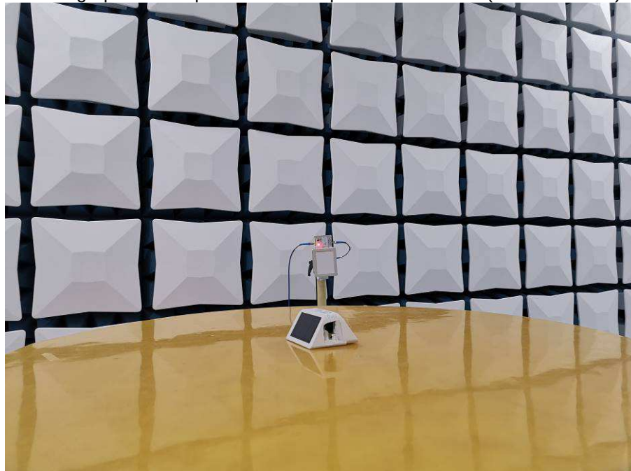
Photograph 2: Set-up for Radiated Spurious Emissions (18GHz-25GHz)
