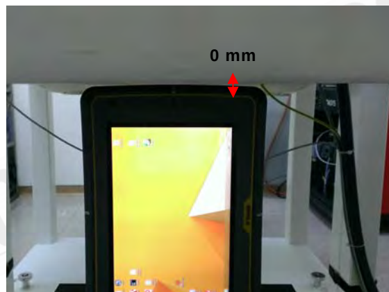
Fig.11 EUT Right side to flat phantom
