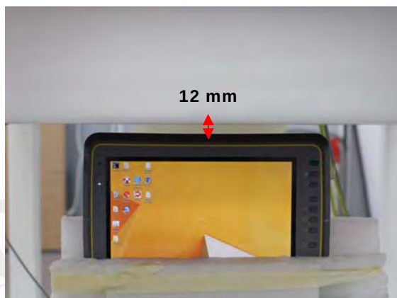
Fig.6 EUT Top side (12mm) to flat phantom
