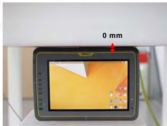
Fig.8 EUT Bottom side to flat phantom
