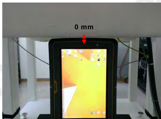
Fig.10 EUT Left side to flat phantom
