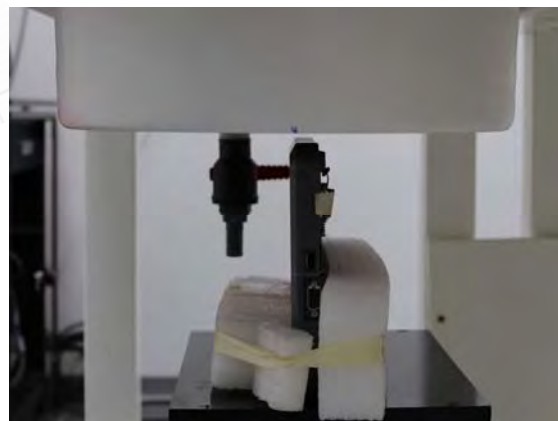
Fig.6 EUT Top side (12mm) to flat phantom
