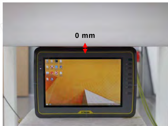
Fig.5 EUT Top side to flat phantom
