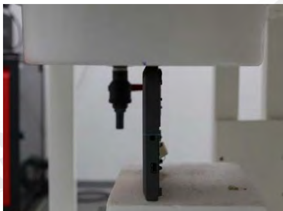
Fig.8 EUT Bottom side to flat phantom
