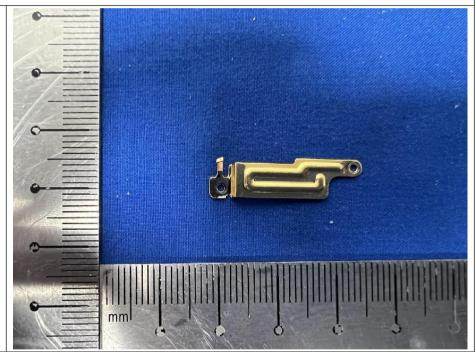
The antenna is PIFA antenna. The best case gain of the antenna is 1.58 dBi.
