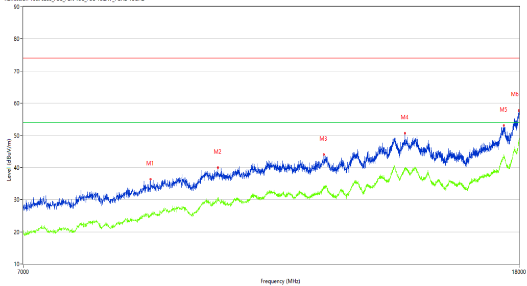
REmission Test case_FCC_Part 15C_FCC 15.247_7GHz-18GHz
