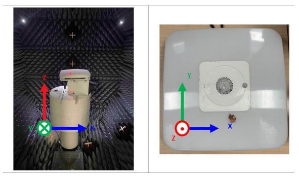
setup photo of BLE antenna:
