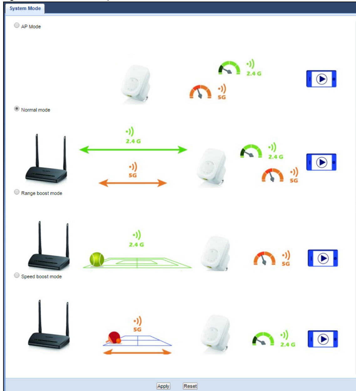
Figure 56 Maintenance > System Mode
