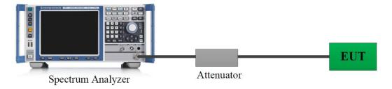
A short RF cable with low cable loss connected to the EUT antenna port, which was provided by manufacturer. The insert loss of this RF cable/attenuator was offset into the setting of test equipment.
