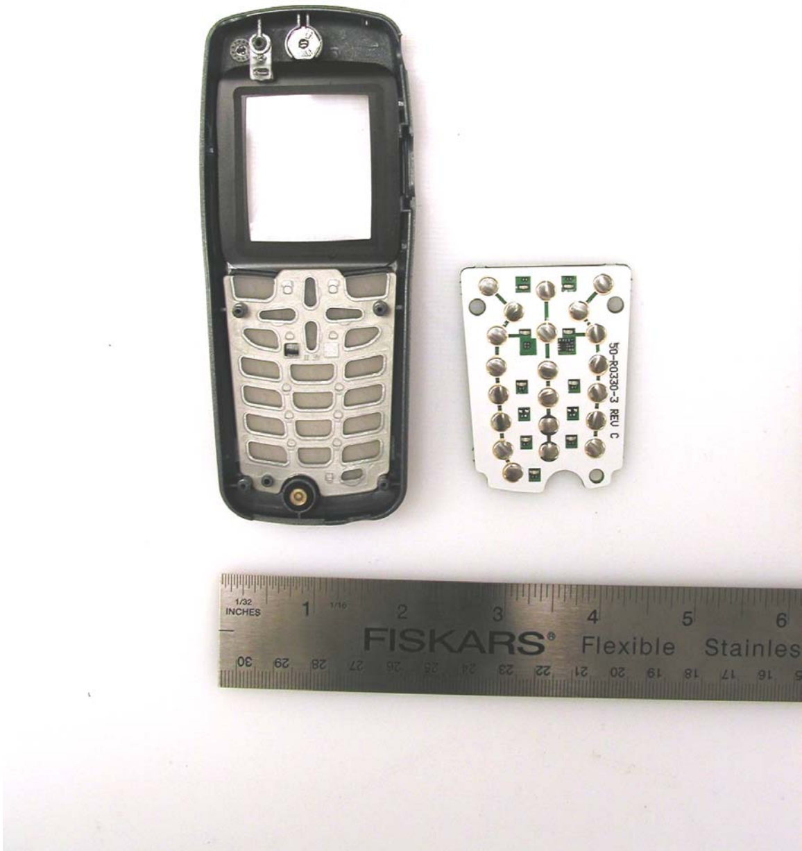
Front housing with keypad printed wiring board removed
