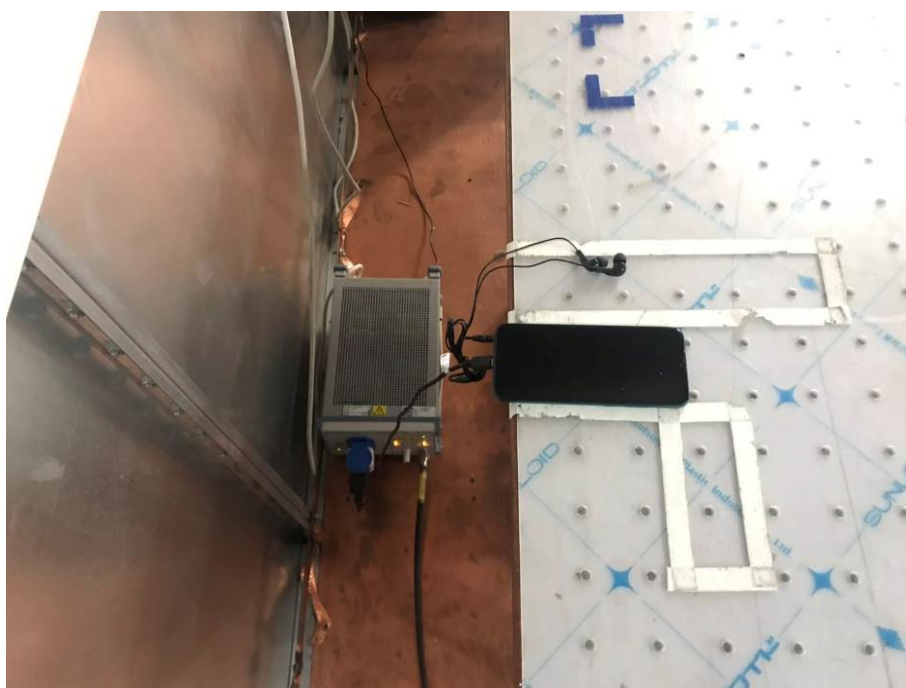
Conducted Emissions Test Setup (with charger)
