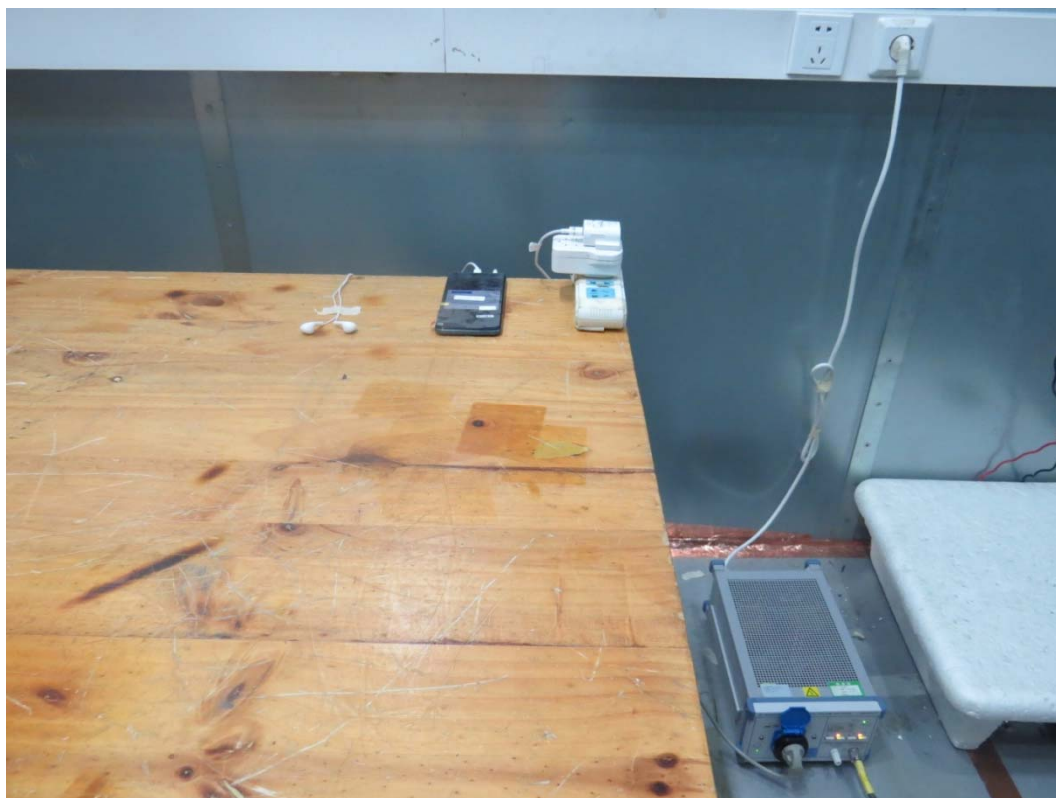
Picture 1: Conducted Emissions Test Setup
