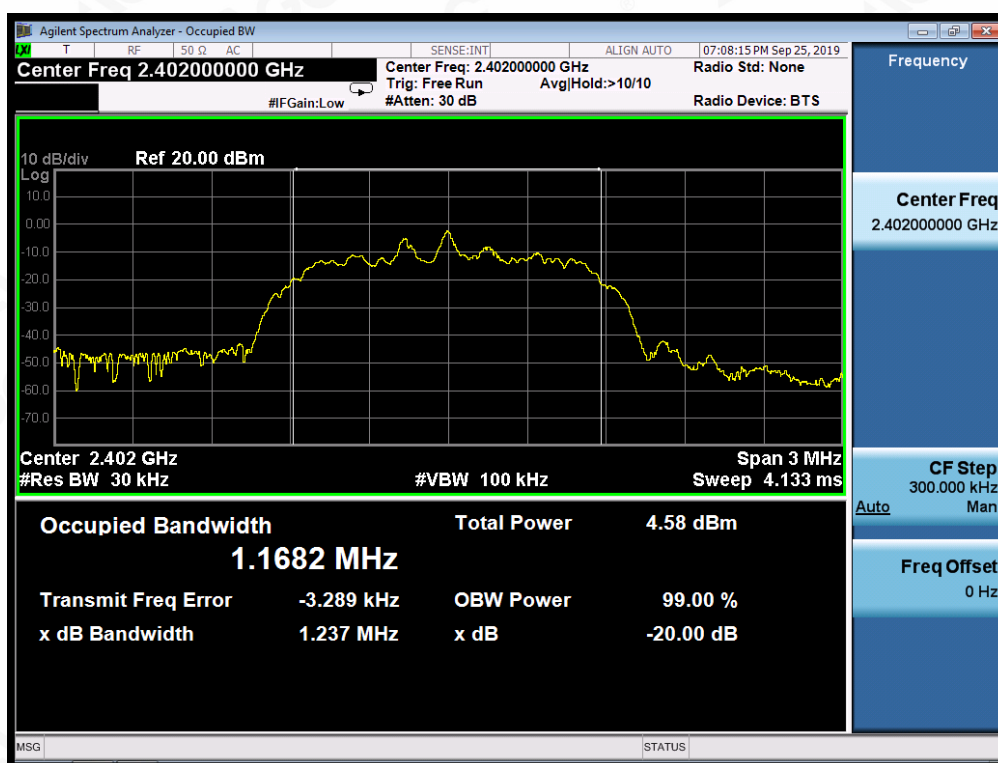
TEST PLOT OF BANDWIDTH FOR LOW CHANNEL
