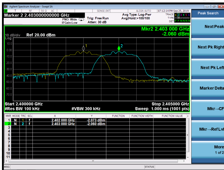
TEST PLOT FOR FREQUENCY SEPARATION
