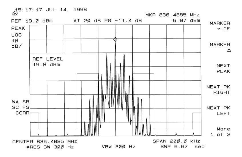
SAT & Signal Tone, Carrier Frequency 836.49 MHz, Power Level 7
