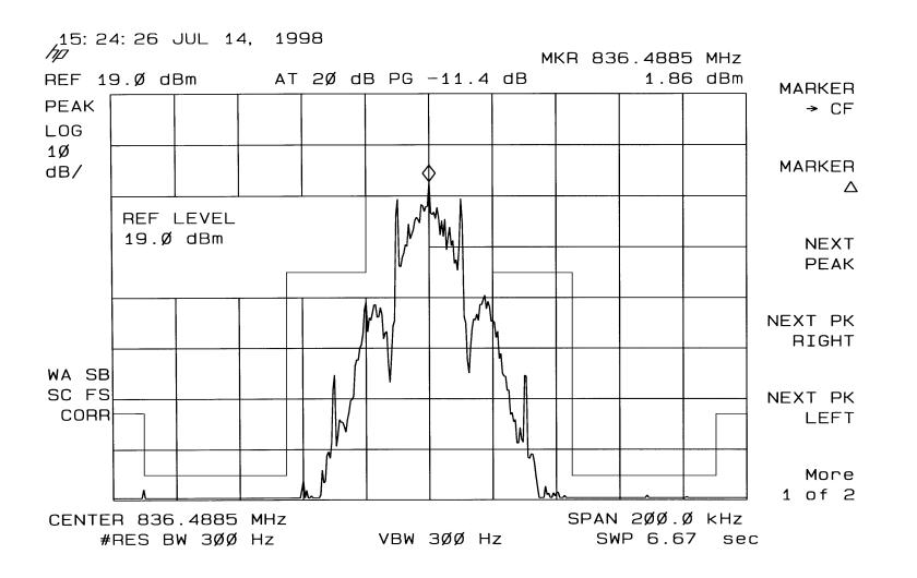
10 kbit/s Wideband Data, Carrier Frequency 836.49 MHz, Power Level 7
