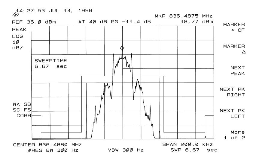
10 kbit/s Wideband Data, Carrier Frequency 836.49 MHz, Power Level 0
