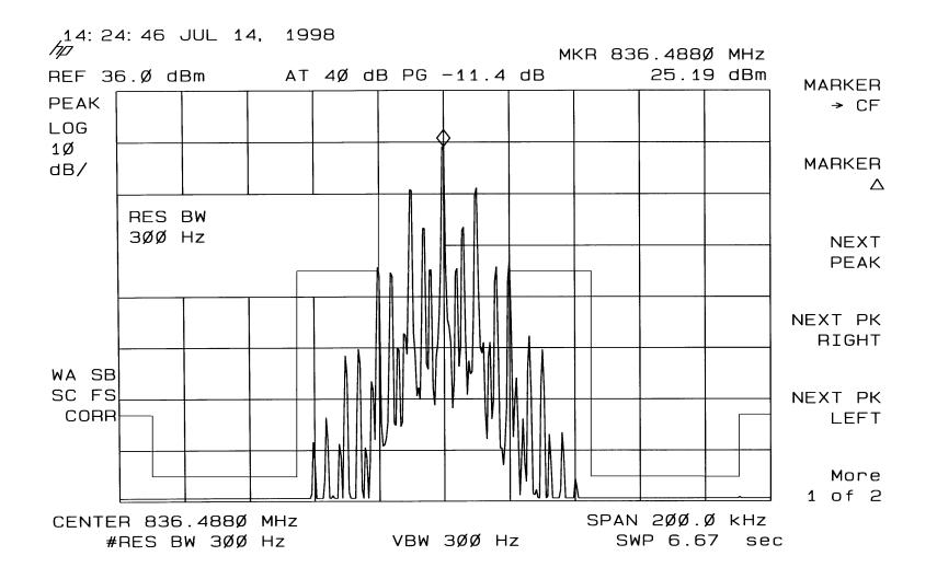
SAT & Signal Tone, Carrier Frequency 836.49 MHz, Power Level 0.
