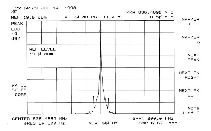
Unmodulated Carrier, Carrier Frequency 836.49 MHz, Power Level 7, Conducted RF Output Power 7.08 mW.
