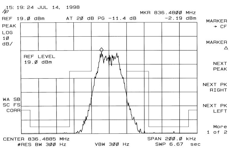
SAT & DTMF #3, Carrier Frequency 836.49 MHz, Power Level 7
