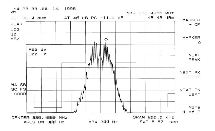
SAT & Voice, Carrier Frequency 836.49 MHz, Power Level 0
