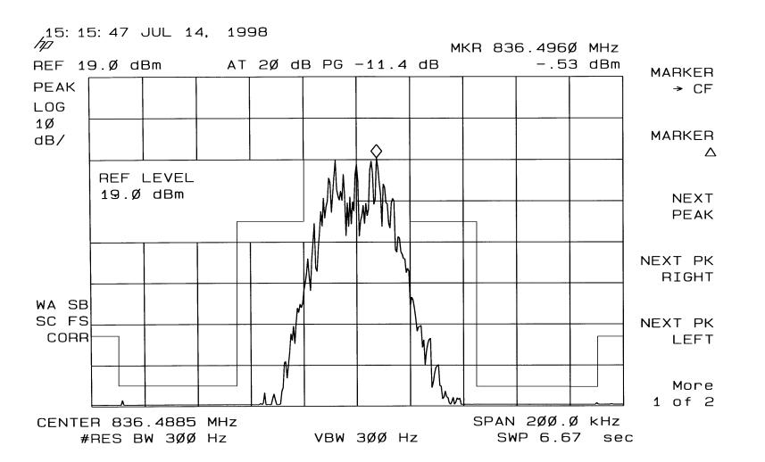
SAT & Voice, Carrier Frequency 836.49 MHz, Power Level 7
