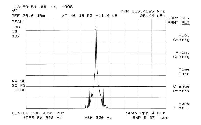
Unmodulated Carrier, Carrier Frequency 836.49 MHz, Power Level 0, Conducted RF Output Power 440.6 mW
