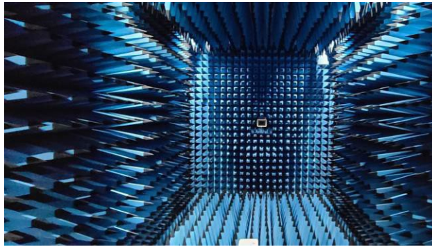
Figure 2: Geometry of Anechoic Chamber for Radiation patterns.
