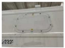
12. Measure 6 cm from the evaporator back panel and place the transceiver bracket onto the evaporator centre plate. Using a pen, mark the position of the 2 holes. Be sure that the 2 holes are in the centre of the plate.
