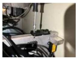
15. Slide the transceiver into the bracket so it clicks into place.
