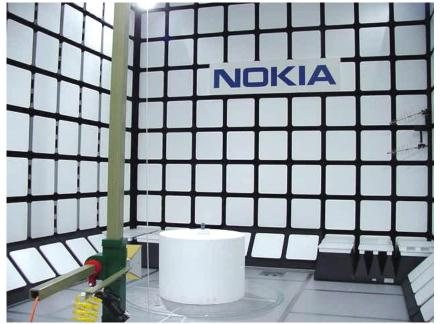
Test method is according to ANSI/TIA/EIA 603A.
